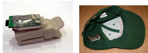
Fig. 22. The wireless PPG finger probe with Bluetooth transmitter, and the “smart” hat with integrated forehead PPG sensor and transmitter [48, 49].
